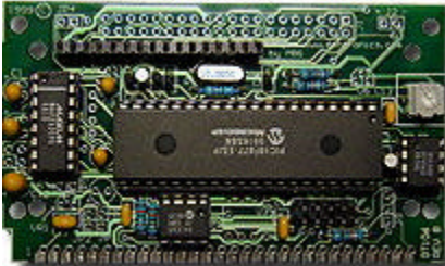
DT106 with 16F877, EEPROM, RTC, RS-232 and LCD
